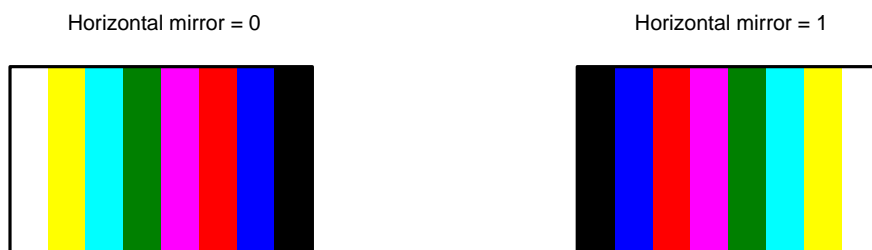
Figure 56. 100% Color Bars Test Pattern
