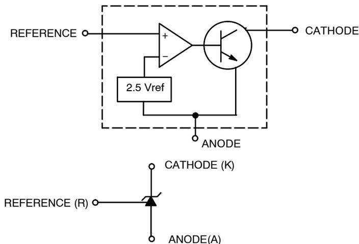
Figure 1. Block Diagram
