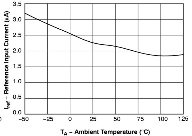
Figure 14. Reference Input Current vs. Ambient Temperature
