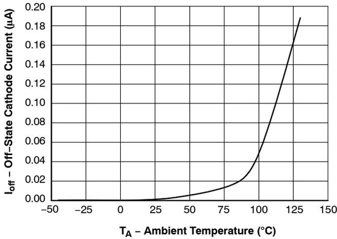
Figure 13. OFF-State Cathode Current vs. Ambient Temperature
