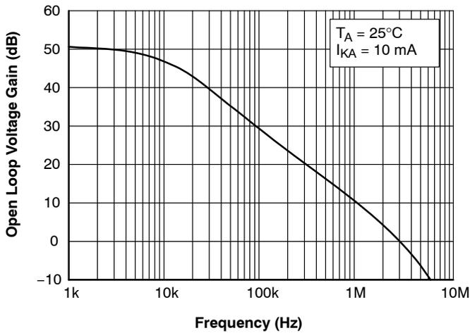
Figure 15. Frequency vs. Small Signal Voltage Amplification
