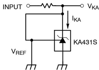
Figure 3. Test Circuit for  $V_{KA} = V_{REF}$
