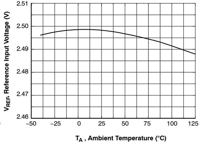
Figure 20. Reference Input Voltage vs. Ambient Temperature
