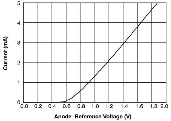
Figure 18. Anode-Reference Diode Curve
