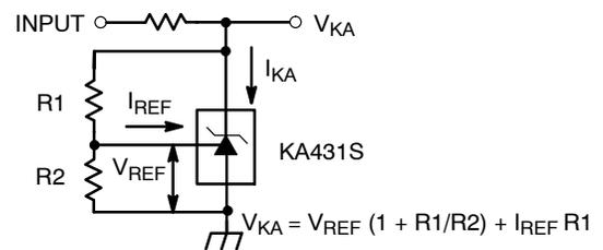
Figure 4. Test Circuit for  $V_{KA} \geq V_{REF}$
