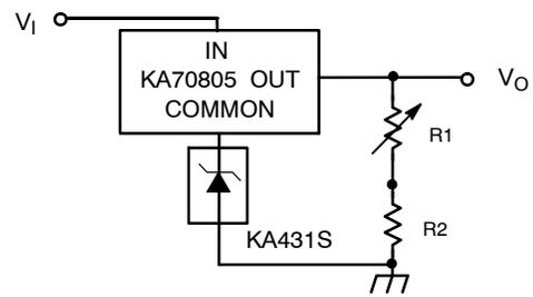
Figure 7. Output Control for Three-Terminal Fixed Regulator
