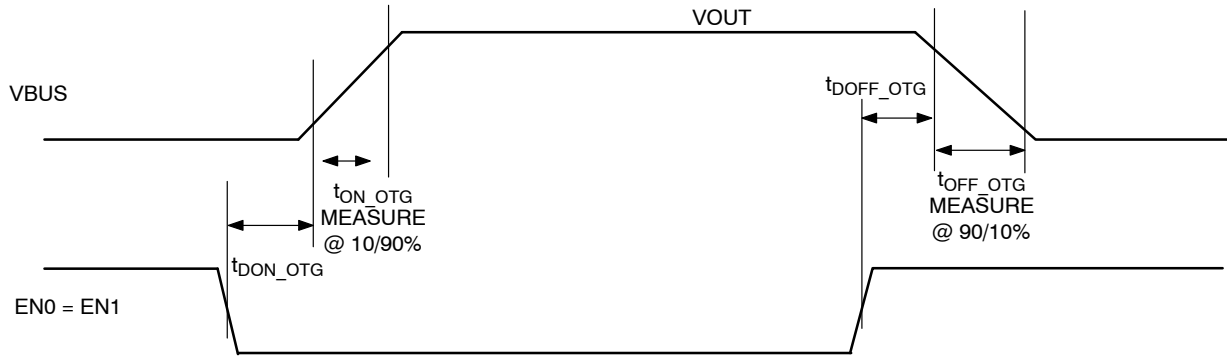
Figure 9. OTG Mode Operation (VOUT = 5 V, VPWR_SIG > UVLO)
