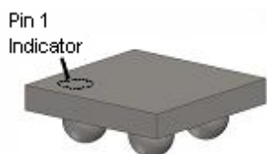
Figure 3. 1 x 1mm WLCSP Bumps Facing Down
