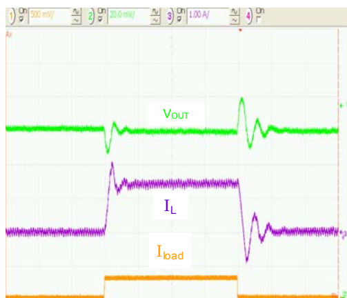
Figure 15. MODE=1, 100 mA to 1.5 A to 100 mA, 5 \mu\text{s}/\text{div} .
