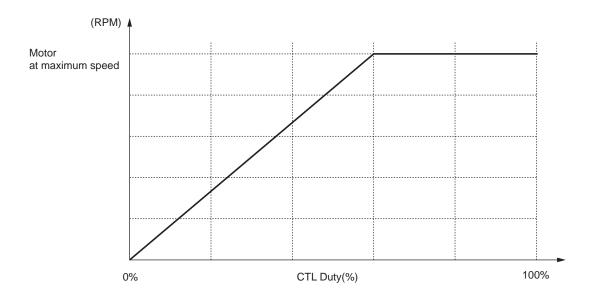
1) Obtain the FG signal frequency fFG (Hz) at the maximum rotational speed of the motor (with two FG pulses per rotation).
