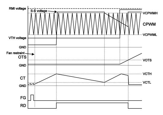
When the fan is constrained, the CT pin voltage rises, and when it reaches VCTH, the lock protection mode is established, and OUTP is set to OFF and RD is set to OFF.
