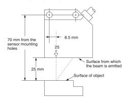
**Note:** Do not tighten the mounting screws for the moment as the optical axis must be adjusted.
