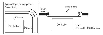
Example: Separating Controller from Power Lines
