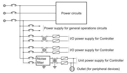
Power Supply System Diagram
