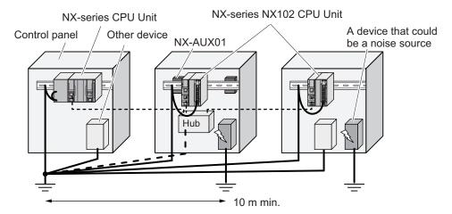
b. Installation by connecting devices and noise sources to a common earth electrode This is an earthing method to connect the device that is connected with a communications cable, other devices, and a device that could be a noise source, to a common earth electrode. This earthing method is not recommended, because the device that is a potential noise source may interfere electromagnetically with other devices.
