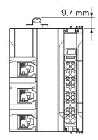
**DIN Track Mounting Hooks** in Unlocked Position
