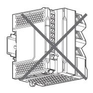
Mounting with the DIN Track Installed Vertically
