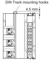
**DIN Track Mounting Hooks** in Locked Position
