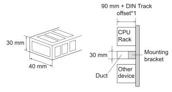
\*1. It varies depending on the DIN Track to be used. Refer to *Installation Dimensions* on page 5-37 under 5-3-12 Assembled Appearance and Dimensions on page 5-37 for details. It corresponds to the dimension (B).
