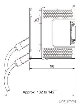
\*1. This is the dimension from the back of the Unit to the communications cables.
