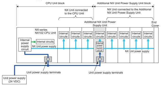
The total of the required Unit power supply capacity for these two blocks is the required power supply capacity of the Unit power supply for the CPU Rack.
