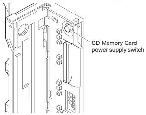
**2** Press the SD Memory Card after you confirm that the SD BUSY indicator (lit while SD Memory Card access is in progress) and SD PWR indicator (lit while SD Memory Card power is supplied) are no longer lit.
