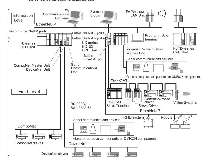
Refer to the *NJ/NX-series CPU Unit Software User's Manual (Cat. No. W501)* for details on the network configuration.
