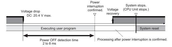
After stopping, the system will restart if the power supply remains recovery.
