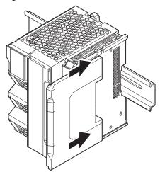
**2** Press the End Cover firmly against the DIN Track until you hear it lock into place on the DIN Track.
