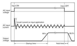
Note: Twice the input current or above will flow during the parallel operation or redundant system. Therefore, check the fusing characteristics of fuses and operating characteristics of circuit breakers making sure that
