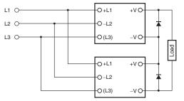
Note: 1. The diode is connected as shown in the figure. If the load is short-circuited, a reverse voltage will be generated inside the Power Supply. If this occurs the product may possibly deteriorate or be damaged. Always connect a diode as shown in the figure.
