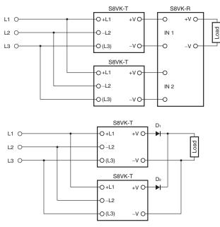
• Use the following information as a guide to the diode type, dielectric strength, and current.
