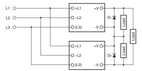
• Use the following information as a guide to the diode type, dielectric strength, and current.
