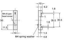
Note: If there is a possibility that the Unit will be subject to vibration or shock, use a steel DIN Rail. Otherwise, metallic filings may result from aluminum abrasion.
