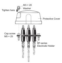
Note: The Protective Cover cannot be mounted on the BF-1.
