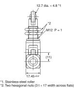
540 gf 114 gf 1.8 mm OF max. RF min. PT max. OT min. MD max. 3.58 mm 0.06 mm OP 33.4±1.2 mm
