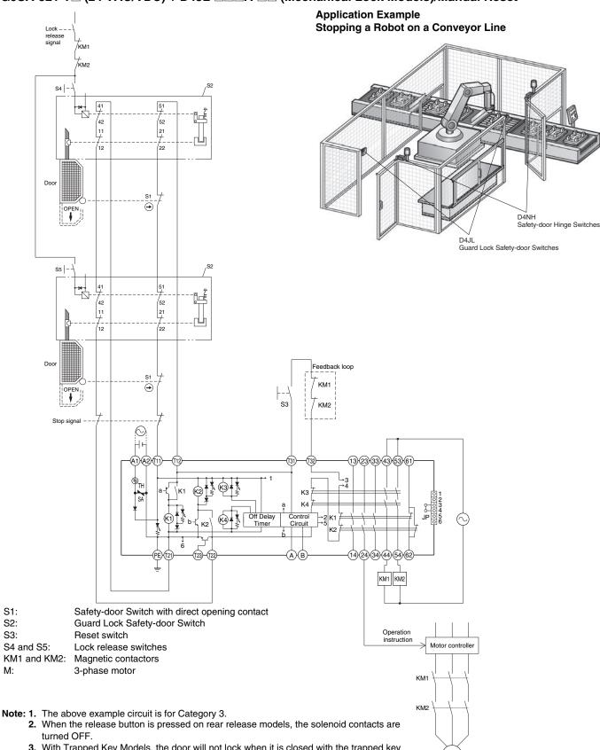
3. With Trapped Key Models, the door will not lock when it is closed with the trapped key removed.
