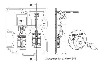
(4) Operation Key inserted, solenoid ON, and trapped key inserted. Status: Door locked and trapped key can be removed.
