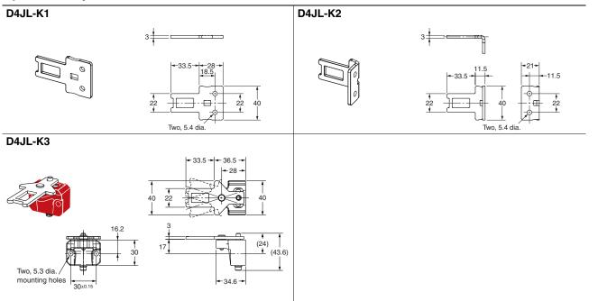
Note: Unless otherwise specified, a tolerance of ±0.8 mm applies to all Switch dimensions and a tolerance of ±0.4 mm applies to Operation Key dimensions.
