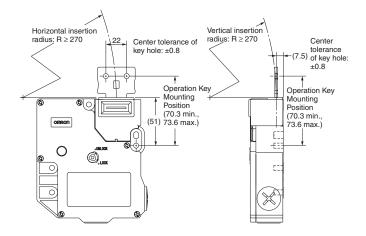
D4JL+D4JL-K2 (with Front-inserted Operation Key)
