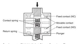
Conforms to EN60947-5-1 Direct Opening  $\bigcirc$ . (Only the NC contacts have a direct opening function.) When contact welding occurs, the NC contacts are separated from each other by pushing in the plunger.
