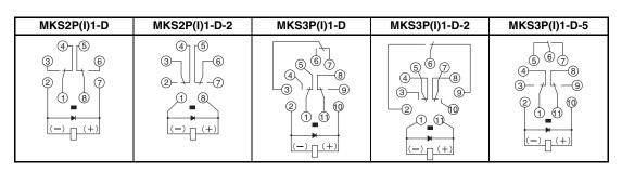
**LED Indicator and** Diode Type (DC Coil)
