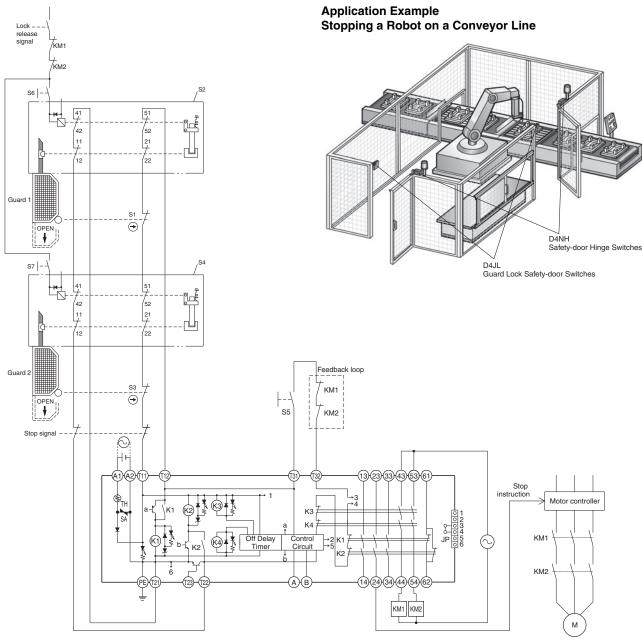
S1: Safety-door Switch with direct opening contact
