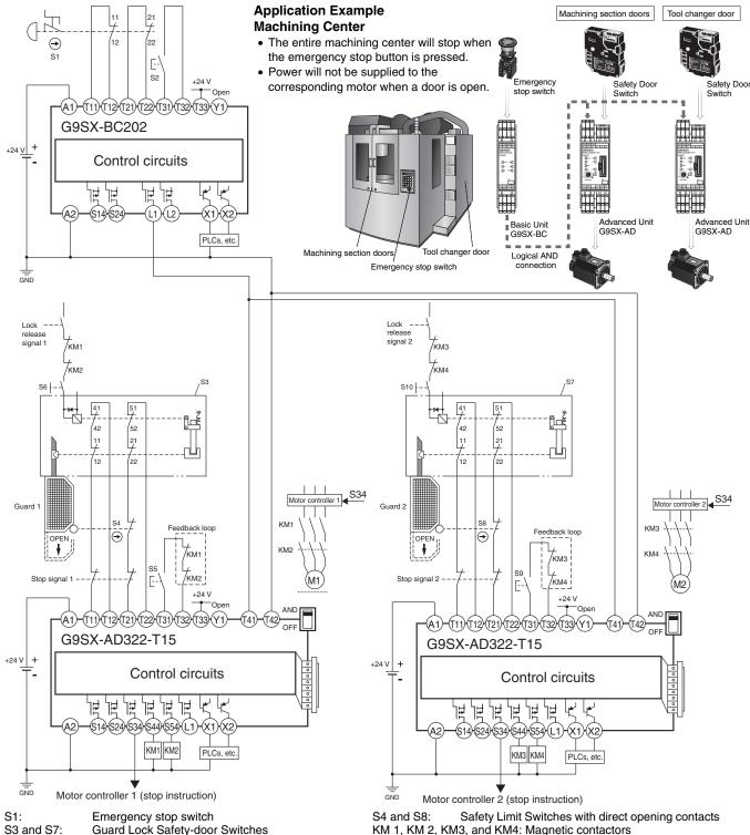
Guard Lock Safety-door Switches S2, S5, and S9: Reset switches
