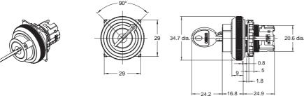
Three-position Switches with Brushed Metal Bezels A30NZ-3M\_-01\_A
