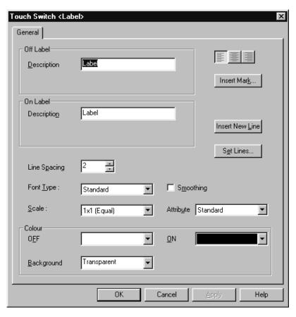
Off Description: Specify the text of the label that will be displayed when lamp bit is OFF.
