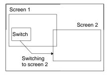
(1) When a touch switch is pressed, the screen is switched to the screen with the specified screen number.
