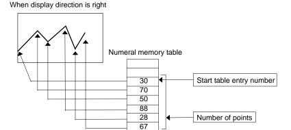
• The intervals between numeral memory table entries in a broken-line graph can be set as even or uneven, as desired, with the [Interval Type] line property.
