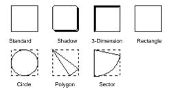
Although [Standard] and [Rectangle] have the same shape, how the touch switch frame is defined differs between them. With [Standard], the touch switch frame itself provides the display graphic. With [Rectangle], however, a rectangle shape can be specified independently of the touch switch frame and the touch switch frame can be separated from the rectangle shape.
