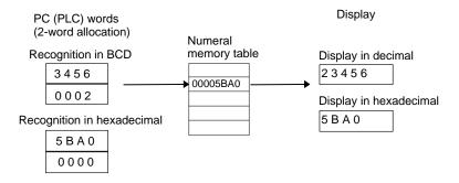
With NT30, NT30C, NT620S, NT620C, and NT625C, the only difference in decimal/hexadecimal display of a numeric value is whether or not F at the most
