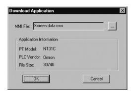
If the PT is not in the Transmit mode, a timeout error occurs in about 10 seconds at the NT Transfer Utility. In this case, set the PT in the Transmit mode and click on set in the error message dialog box.
