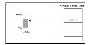
(1) A value in a numeral memory table entry is converted into a percentage value, in the range from 0 to 100% or from –100% to 100%, and displayed in the form of a bar graph.
