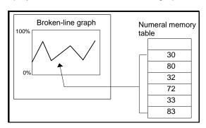
(1) The values of consecutive memory table entries are converted into percentage values, in the range from 0 to 100% or from –100% to 100%, and displayed in the form of a broken-line graph.
