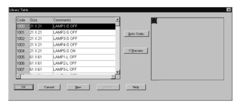
(2) If the code of the desired library data is not found in the list, scroll the list using the scroll bar at the right side of the screen, or click on Goto Code. to open the code input dialog box.
