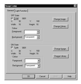
To display the image data or the library data only when the PC (PLC) bit is ON or OFF, cancel the check mark in the check box of the bit status for which the image/library data is not to be displayed.
