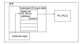
The extended I/O input table notifies the PC (PLC) of the status (ON/OFF) of the input terminals.
