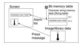
(1) When the bit memory table entry number in the specified range goes ON, the alarm list element reads out the alarm message from the character string memory table entry (string table) and displays the message at the alarm list area in the screen.
