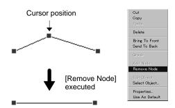
• To remove a vertex, locate the cursor on the vertex to be removed and select [Remove Node] in the pop-up menu.
