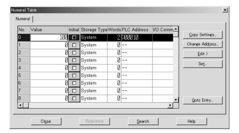
(2) If the number of the desired numeral table entry is not found in the list, scroll the list using the scroll bar at the right side of the screen, or click on
