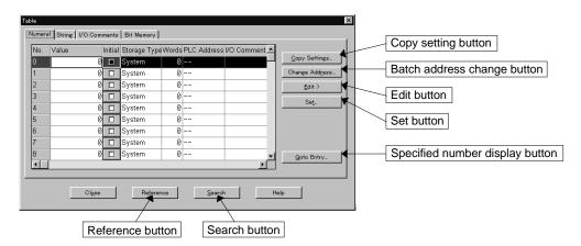
Operation starts by specifying the number, that is, clicking on the objective line (memory table entry number). The shape of the mouse cursor changes as shown below when it enters the No. field.
