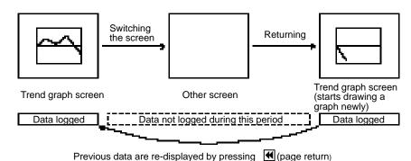
The trend graph is drawn newly when the screen is switched back to the trend graph display screen. However, it is possible to redisplay the past data drawn in the trend graph previously by pressing a touch switch that has the function to display the past data. In this case, however, the data are not logged while a trend graph is not displayed.
