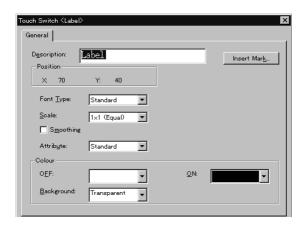
For the procedure for setting the properties, refer to *6-2-7 Text*. When using the NT21, NT31, NT31C, NT631, and NT631C, it is possible to set different colors for the lamp ON and lamp OFF states. With these models, however, it is not permissible to insert image data.
