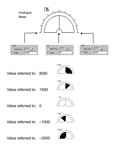
If the 100% value, 0% value, and –100% value are set using numeral memory table entries as indicated below, the percentage value of the reference value is calculated according to the value stored at the specified address.
