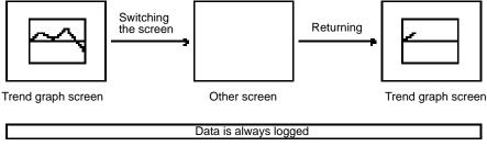
Although the trend graph starts displaying new data when the screen is switched back to the trend graph display screen, it is possible to display the data of the period during which the trend graph was not displayed by pressing a touch switch that has the function to display the past data.
