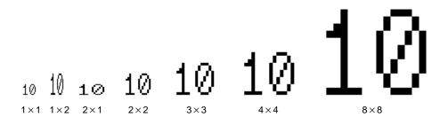
**Reference:** With the NT21 and with the NT31, NT31C, NT631, and NT631C "-V1" and above, numbers of 2×2 or larger scale are automatically displayed in 32 dot font.
