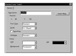
For the procedure for setting the properties, refer to *6-2-7 Text*. For the NT21, NT31, NT31C, NT631, and NT631C, it is possible to set different colors for lamp ON and lamp OFF by setting [Color – OFF] and [Color – ON] instead of setting label color. However, background color is fixed to transparent for the NT21, NT31, NT31C, NT631 and NT631C.
