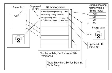
An alarm list element is used in combination with bit memory table entries. How they function is shown below:
