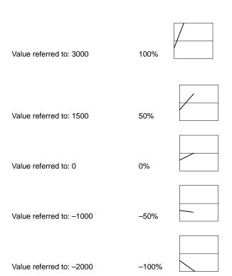
If the 100% value, 0% value, and –100% value are set using numeral memory table entries as indicated below, the percentage value of the reference value is calculated according to the value stored at the specified address.
