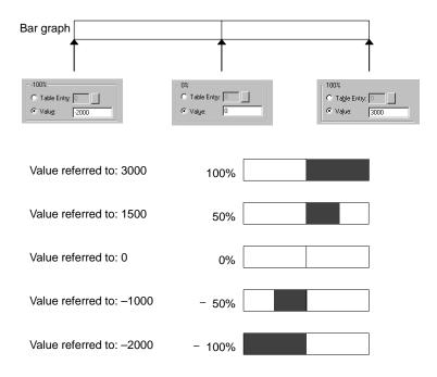
If the 100% value, 0% value, and –100% value are set using numeral memory table entries as indicated below, the percentage value of the reference value is calculated according to the value stored at the specified address.
