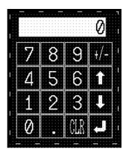
(1) Move the range specifying frame, displayed at the upper left section in the screen, to the numeric key area and adjust its size so that the keys and temporary input field are enclosed.
