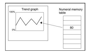
(1) The value in a numeral memory table entry is converted into percentage values at the set intervals, in the range from 0 to 100% or from –100% to 100%, and displayed in the form of a trend graph.
