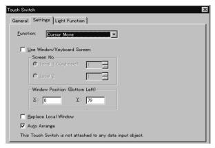
If a check mark is set for [Use Window/Keyboard Screen] in the cursor moving touch switch setting properties, it is possible to display the specified window/ keyboard at the same time the cursor is moved.
