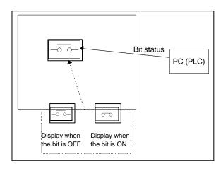
(1) The image data or the library data is switched to be displayed according to the status of the allocated PC (PLC) bit.
