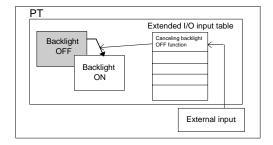
When the input terminal goes ON, the backlight, which has been turned OFF by the Cancel Backlight Off function set by a memory switch, is turned ON to redisplay the screen. A backlight OFF function releasing attribute is automatically provided for the screen switching function and the control code input function.
