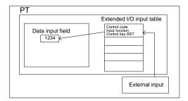
When the input terminal goes ON, it has the same effect as pressing of the control key.
