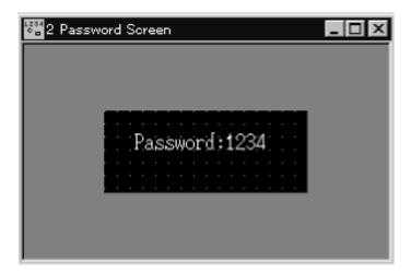
The figure above shows a new password screen created. It has a text element with "password" as labeled. Next to the text element is the password element that indicates the current password for this password screen. In the password property page, you can set the password and the designated screen number to be displayed next.
