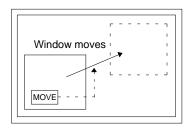
(1) When a touch switch (window move touch switch) is pressed, the window can be moved by touch panel operation at PT. When you press the destination (center of the window will come here), window will be moved to that position.
