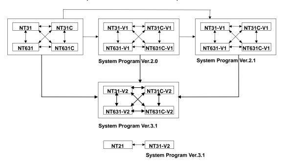
It is possible to convert the screen data for the lower system program version to that for the higher system program version freely regardless of the PT models. (e.g., from "-V1" to "-V2" or from "-V2" to "-V2 (System Ver3.1)).
