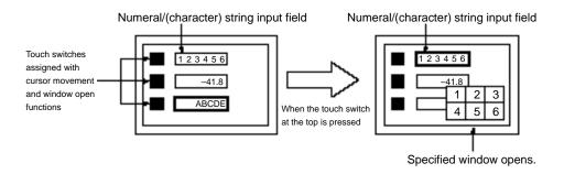
**Reference:** • A cursor moving touch switch can be created automatically when creating a numeral input element or a (character) string input element.
