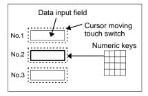
If a touch switch on input field No. 2 is pressed, the No. 2 input field becomes the objective field for data input. The data input using the numeric keys is stored in input field No. 2.
