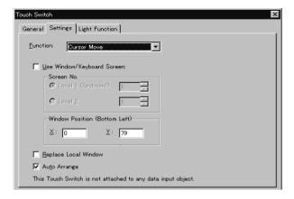
If a check mark is set for [Use Window/Keyboard Screen] in the cursor moving touch switch setting properties, it is possible to display the specified window/ keyboard at the same time as the cursor is moved.
