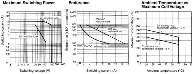
Note: The maximum coil voltage refers to the maximum value in a varying range of operating power voltage, not a continuous voltage.
