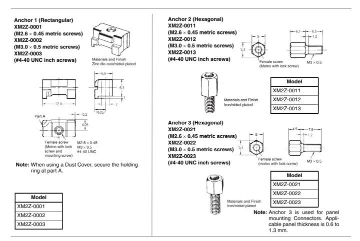
Note: 2 anchors are necessary per connector.
