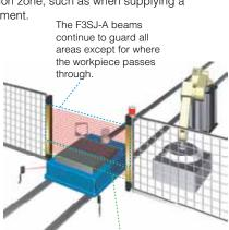
Only the beams of the safety light curtain interrupted by the workpiece are muted.
