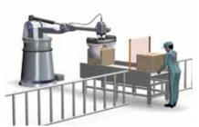
is performed. A limit switch or other means is used to detect when the robot is in a safe position and muting is then applied.
