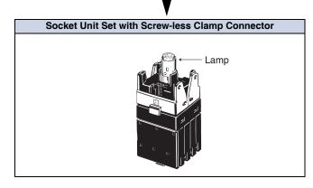
Ordering as a Set ...... The model numbers used to order sets of Units are given in the following tables. One set comprises the Display, Case, Lamp, and Socket.
