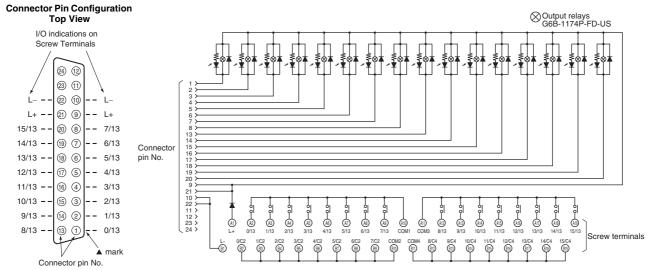
**Note:** Pin numbers are indicated for convenience. The ▲ mark can be used to determine orientation.
