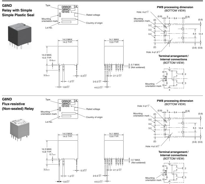
\* Tolerance unless otherwise specified Less than 1 mm: ±0.1 mm Less than 1 to 3 mm: ±0.2 mm 3 mm or more: ±0.3 mm
