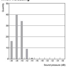
Sample: G5RL-1A-LN 12 VDC Number of relays: 100 pcs Range: A weighted sound pressure level,
