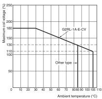
Note. The maximum coil voltage refers to the maximum value in a varying range of operating power voltage, not a continuous voltage.
