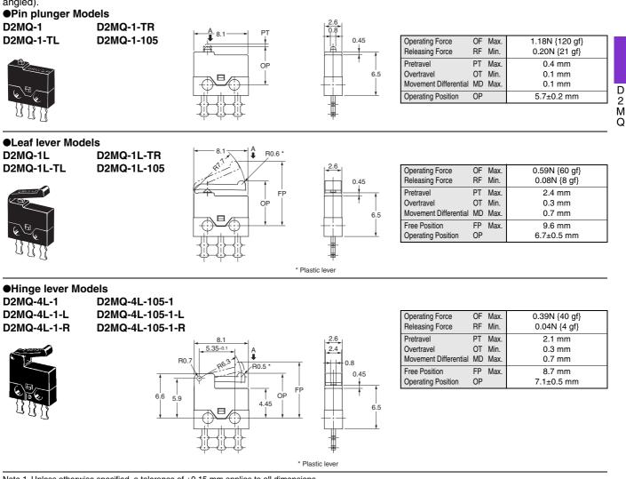
Note 1. Unless otherwise specified, a tolerance of  $\pm 0.15$  mm applies to all dimensions. Note 2. The operating characteristics are for operation in the A direction ( $\clubsuit$ ).
