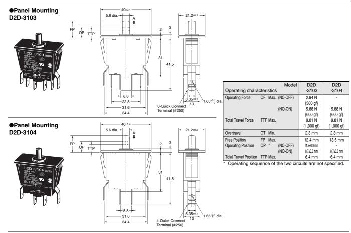
Note 1. Unless otherwise specified, a tolerance of ±0.4 mm applies to all dimensions. 2. The operating characteristics are for operation in the A direction (  $\clubsuit$  ).
