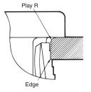
When processing the panel, be sure that the Play R is on the switch operation side. Be sure that the Edge is on the reverse side of panel when processing.
