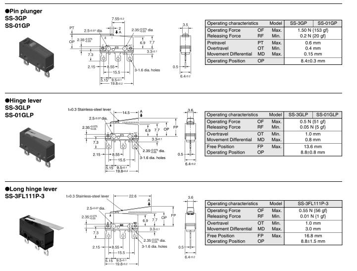
Note 1. Unless otherwise specified, a tolerance of  $\pm 0.4$  mm applies to all dimensions. Note 2. The operating characteristics are for operation in the A direction (  $\clubsuit$  ).
