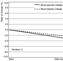
Characteristics were measured after applying vibration at a frequency of 10 to 55 Hz (single amplitude of 0.75 mm) to the test piece (not energized) for 2 hours each in 3 directions. The percentage rate of change is the average value for all of the samples
