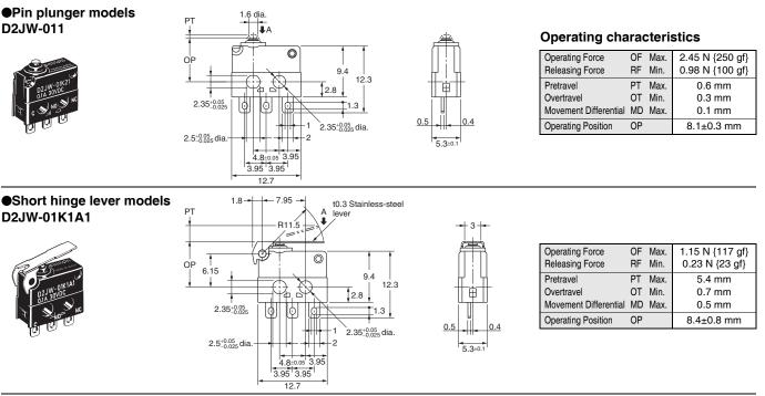
Note 1. Unless otherwise specified, a tolerance of ±0.4 mm applies to all dimensions. Note 2. The operating characteristics are for operation in the A direction ( I).
