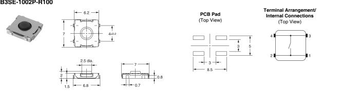
Note: Unless otherwise specified, a tolerance of ±0.4 mm applies to all dimensions. No terminal numbers are indicated on the Switches.
