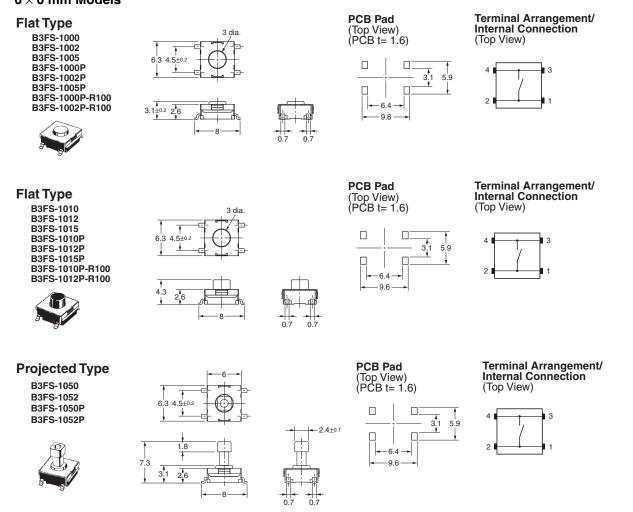
Note: Unless otherwise specified, a tolerance of ±0.4 mm applies to all dimensions. No terminal numbers are indicated on the Switches.
