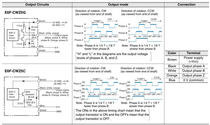
Note: 1. The shielded cable outer core (shield) is not connected to the inner area or to the case.
