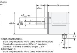
(Conductor cross section: 0.2 mm², Insulation diameter: 1.0 mm), Standard length: 0.5 m
