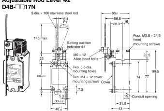
Note: Unless otherwise specified, a tolerance of  $\pm 0.4 \ \text{mm}$  applies to all dimensions.
