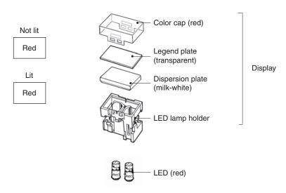
Colored illumination describes LED models for which the screen color is white when the LED is not lit and changes to the color of the LED lamp when the LED is lit.
