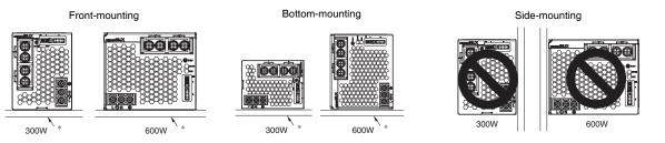
Note: 1. Improper mounting will interfere with heat dissipation and may occasionally result in deterioration or damage of internal parts. Use the standard mounting method only.
