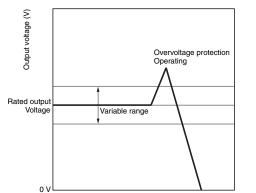
Note: Do not turn ON the power again until the cause of the overvoltage has been removed.
