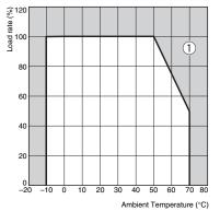
Note: 1. Internal parts may occasionally deteriorate or be damaged. Internal parts may occasionally deteriorate or be damaged. Do not use the Power Supply in areas outside the derating curve (i.e., the area shown by shading ① in the above graph).
