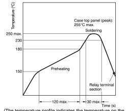
(The temperature profile indicates the temperature on the PCB.)
