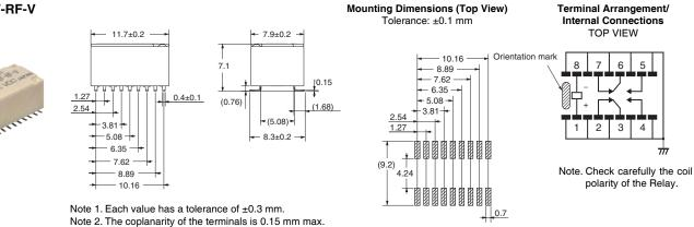
Note 3. The dimensions of the printed circuit board work drawing are a recommended example that take soldering into consideration. Frequency characteristics vary depending on the band dimensions, so check the effect on high-frequency characteristics using a test board before use.
