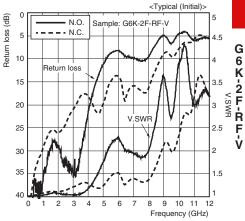
Note 1. The high-frequency characteristics depend on the mounting board. Be sure to check operation including durability in actual equipment before use. Note 2. Ambient temperature condition: 23°C.
