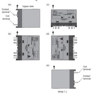
Note 1. The operating voltage differs from the applied coil voltage for contact terminals mounted in the downward direction (e). Please refer to Coil on page 1 and •Relay Operation and Coil Voltage Reduction (Holding Voltage).
