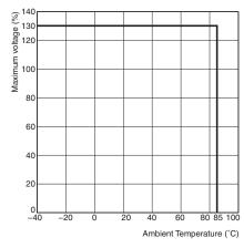
Note. Maximum voltage of set pulse and reset pulse at duty factor 10%.
