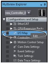
2 Select the I/O port on the I/O Map Tab Page and enter the variable name in the Variable Column.
