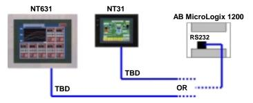
An alternative cable configuration uses a custom RS-232 9-to-9 PIN cable connecting to the Allen-Bradley 1767-CBL-PM02(Series C). The diagram below shows the pinouts for the custom RS-232 cable:
