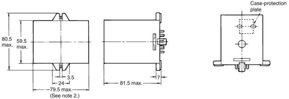
Note 1: As shown in the diagram, there are three 10-dia. holes in the side of the case for MM□XP(N, -D).
