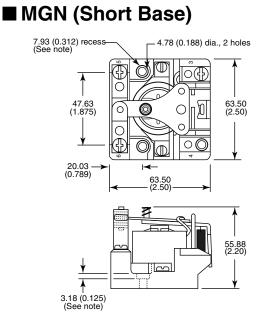
Note: Recess for screw mounting on units with 300-600 VAC coils
