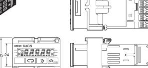
The K3GN uses M3 terminals. A terminal cover is provided.
