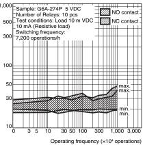
The tests were conducted at an ambient temperature of 23ºC. \*2. The contact resistance data are periodically measured reference values and are not values from each monitoring operation. Contact resistance values will vary according to the switching frequency and operating environment, so be sure to check operation under the actual operating conditions before use.
