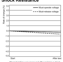
Characteristics were measured after applying a shock of 490 m²/s to the test piece 3 times each in 6 directions along 3 axes. The percentage rate of change is the average value for all of the samples.
