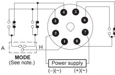
**Note:** The output contact can be set to either instantaneous or time-limit contact using the output type selector located at the upper right corner of the front panel.
