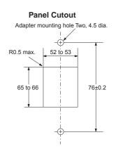
**Dimensions with Y92F-71 Flush Mounting Adapter**
